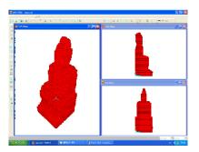
Figure 3. 3D FEM of a typical Nemrut monument
